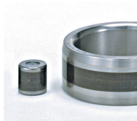
Fig. 4-2 Electric pitting generated on general purpose bearings (pits)
